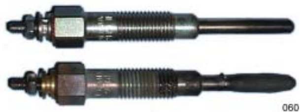
Fig. 9: Intact glow plug (above) and damaged glow plug in short circuit (below).
