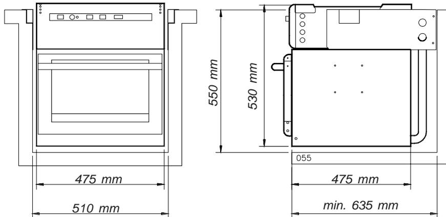
Figure 6: The dimensions of the space required for installation of the 96 D oven's control panel. Heat will make electronics life time shorter; It is not recommended to mount the control panel right above the shutter of the oven.
