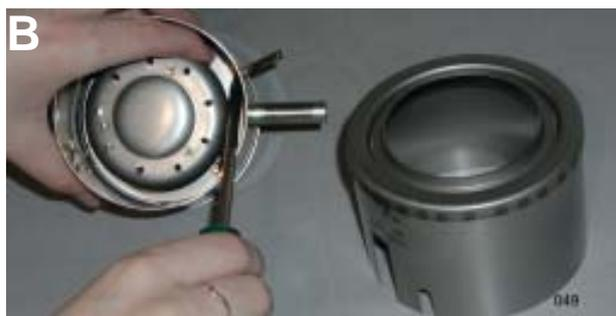
9. If the bottom carpet remains intact, it can be re-used; otherwise, it must be replaced with a new one. The bottom carpet must be intact at least under the glow plug.
