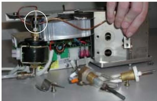
6. Open the bottom of the combustion chamber by removing the two nuts. Pressed against the bottom is a spring, which keeps the burner cylinder in place. Figure 17 a. Pull the burner cylinder out of the burner chamber.
