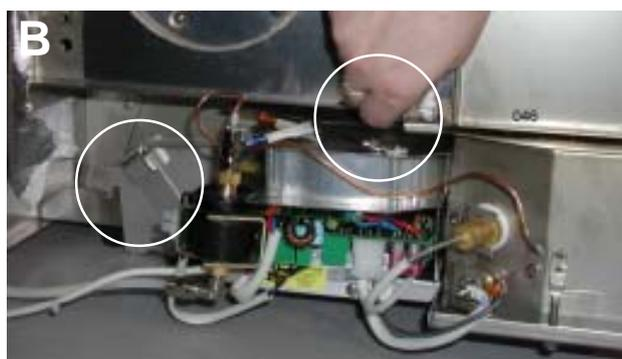
4. Remove the glow plug, the burner temperature sensor and fuel needle by opening the fastener screws and pulling the parts out of the burner. Figure 16.
