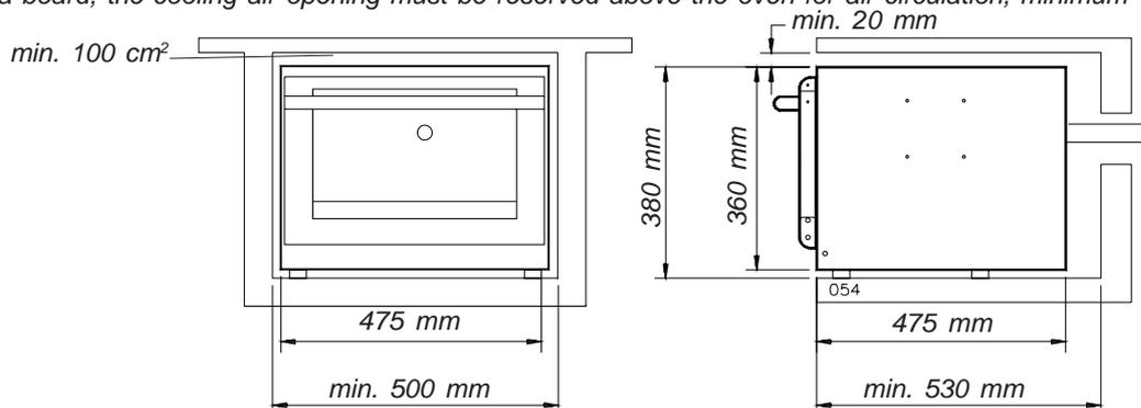
Figure 5: Minimum dimensions of the space required for installation of stove. When installing the stove into a fixed position, the width and depth measurements of the installation opening are identical to those shown in the oven installation diagram 495 mm and 530 mm. Figure 4. When installing a gimbal-mounted oven, the width and depth measurements of the installation opening are identical to those shown in the installation diagram for the stove 510 mm and 550 mm. Figure 5.
