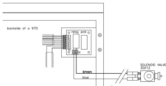
If solenoid valve must be installed to the fuel system, it must open when one or both appliances are used. 97D oven-stove unit has in build a relay pcb. Install solenoid valve wires to connection C2. Solenoid valve uses always two wires; these wires are included in the solenoid valve kit 30012.
