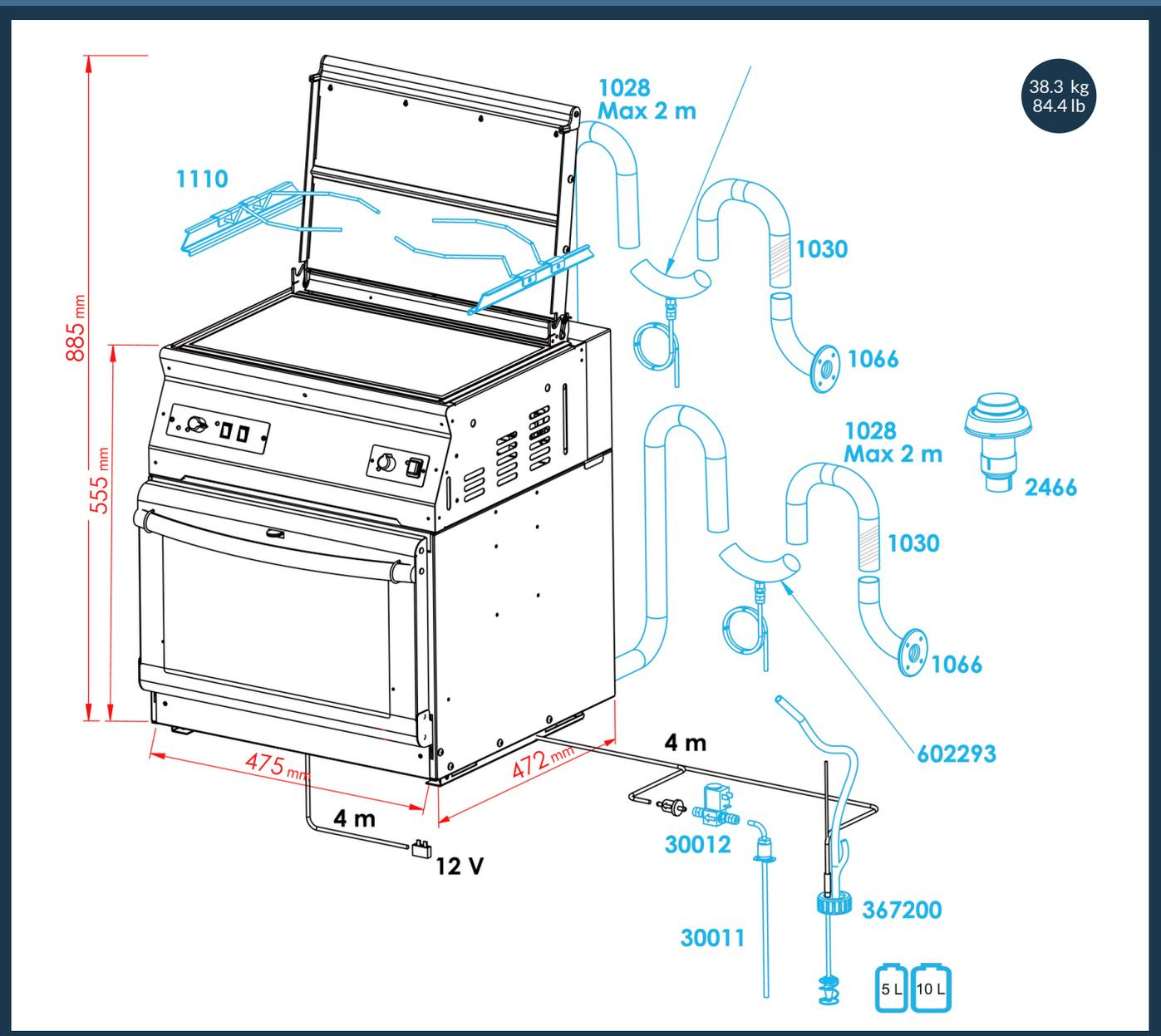
Accessories in black come with the standard package. Accessories in blue are additional/optional. The calculated values are measured in a reference measurement wall, which is constructed to represent a typical boat installation. The figures allow for 10% reserve - yours may vary.
